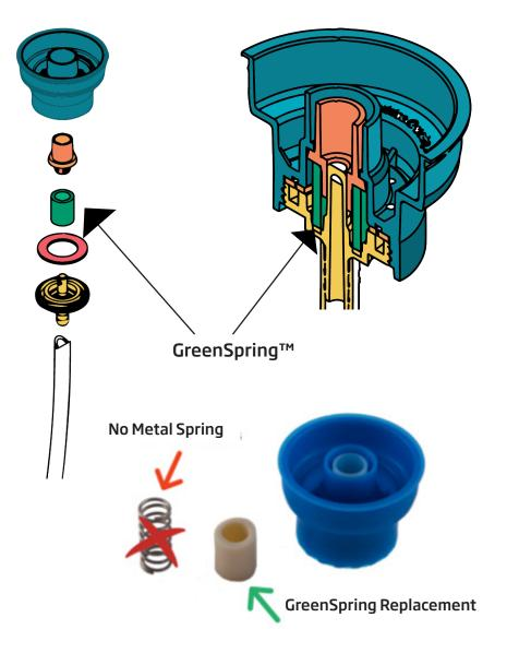
The GreenSpring<sup>™</sup> (*patent pending*) is a revolutionary replacement for metal springs manufactured from TPE.
