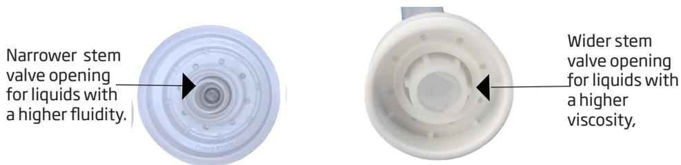
Narrower stem valve opening for liquids with a higher fluidity.
