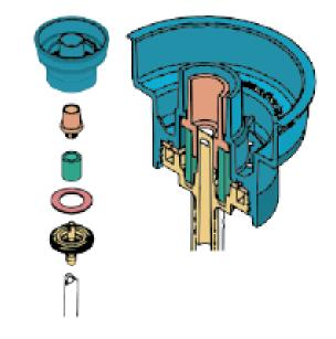
The GreenSpring<sup>™</sup> is manufactured from TPE and is a revolutionary replacement for the metal spring. By replacing the metal within our SafTflo bottle inserts, we are able to offer a superior product that is sustainable manufactured with wider chemical compatibility.
